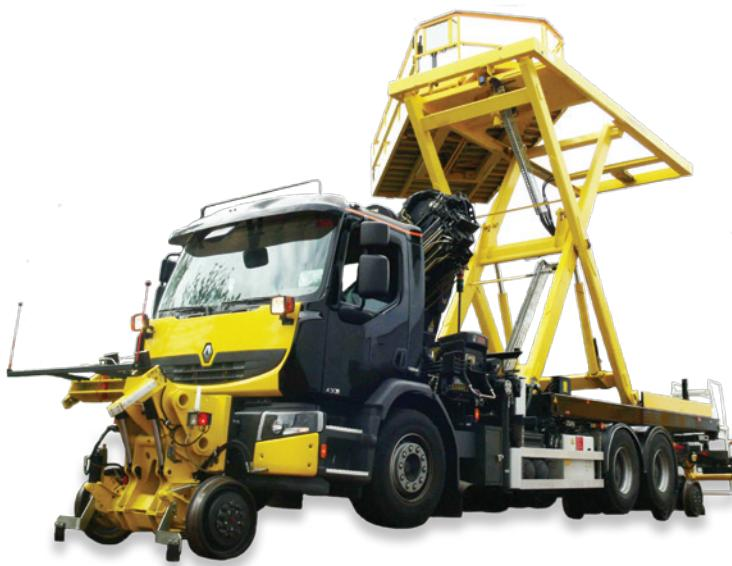
The concept of the X-RAILER 6x4 chassis enhances productive outputs using a variety of modular equipment options mounted on a base unit for an easy on/off tracking and provides safe access when constructing or renewing railway catenary networks. This combination with the NEOTEC's hydrostatic railway driveline, provides the X-RAILER with the best in terms of rail stability with exceptional carrying capacity.
