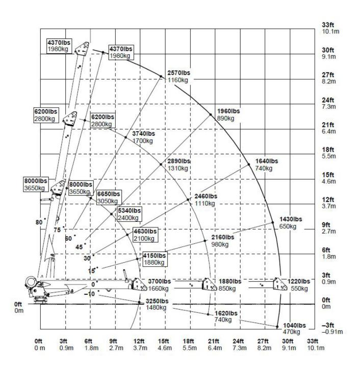
Weights of load-handling devices are part of the load lifted and must be deducted from the capacity.
