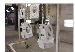
**TOP COAT** For all non-black crane components, a top coat polish is applied to certify maximum durability and finish.
