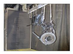
**MEDIA BLAST** A high quality exterior protection that removes any surface imperfections and provides an optimized surface for E-Coating.
