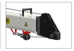
**LOAD BLOCK STOWING BRACKET** Bracket and pads designed to keep load block from contacting the boom when stowed.
