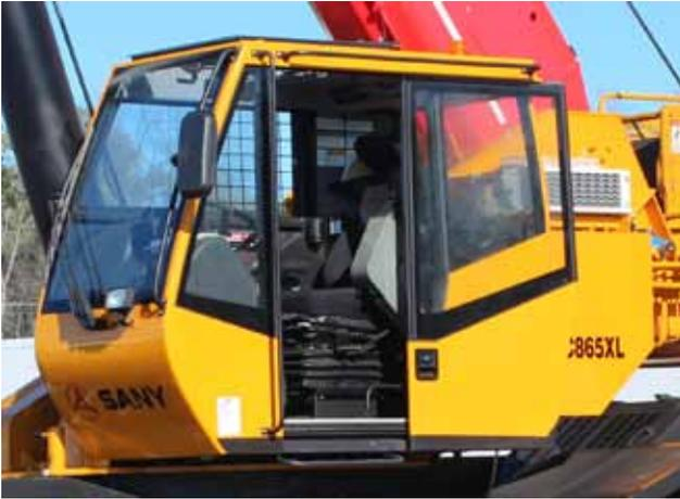
Spacious ergonomic cab with all steel construction. Optimum visibility, tinted safety glass throughout. Opening skylight with visor and wiper system. Sliding door on the left hand side and a framed sliding window on the right hand side. Acoustical foam to absorb noise and insulate the cab. Deluxe six-way adjustable seat is equipped with mechanical suspension and includes arm rests and head rest.
