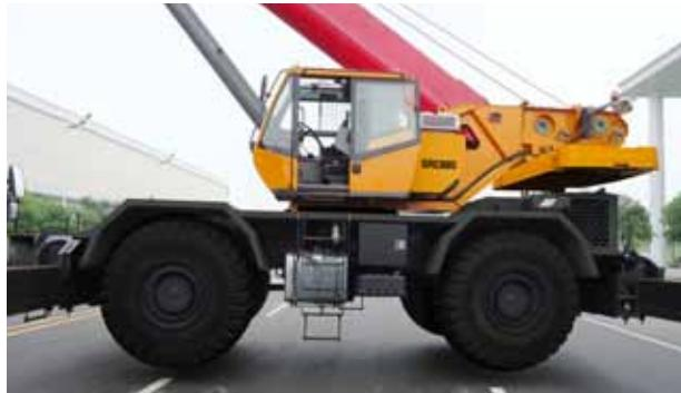
The 275 hp Cummins Tier 4i engine is perfectly integrated with the hydraulic system to deliver precise control and multi-function load sharing. Hydraulic joysticks give the operator smooth, variable control of crane functions. The two-speed swing system can continuously rotate 360 degrees in either direction.
