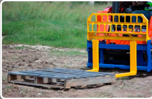
Pallet Forks for skidsteer loaders are not only for the use inside, but also ideal for the uneven grounds of a construction site
