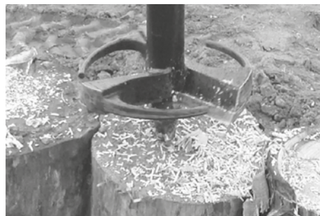
The unique pilot is drilling into the surface of the tree stump and pulling down the planer unerringly.
