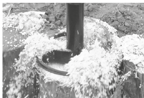
The cutters are trimming the stump with each turn and plane off the wood in splints.
