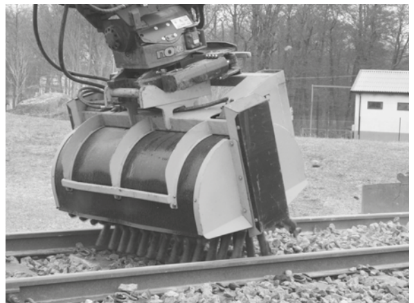
The SKB-Ballast without skirts of protection (in Sweden) shows better how the ballast brush works
