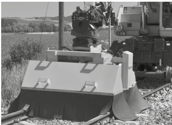
Safer working on the track: A SKB-Ballast with protection skirt made from rubber
