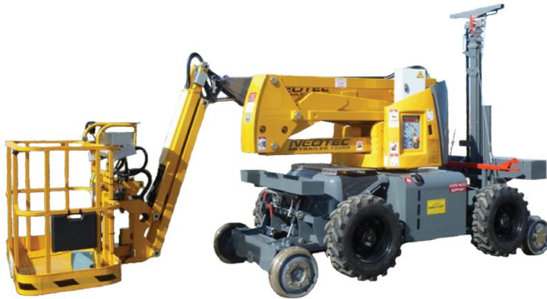
The SKYRAILER 120RR is a versatile vehicle enabling operation on different types of railway networks (Rail, Tramway, Underground).
