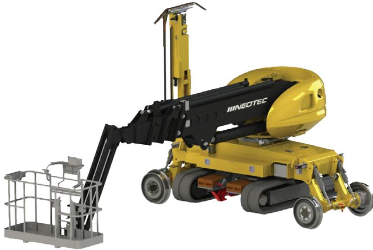
The SKYRAILER 300C RR is the result of NEOTEC expertise on the MEWP market. A special telescopic platform has been developed to reach the catenary as close as possible. The tracks give the operators an easy on-tracking for all kind of fields.
