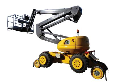
The SKYRAILER 400RR has been developed by NEOTEC in co-operation with Manitou on their 160ATJ+ Aerial Work Platform. The NEOTEC HI-RAIL EPV 14.32 axles guarantee safety in operation on rail and during on or off tracking. The only MEWP of its class offering full 400 kgs payload throughout its whole working envelope.
