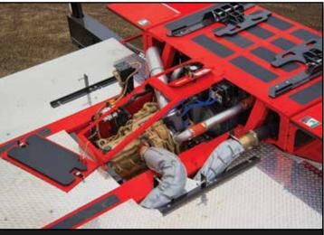
Swing-out doors provide exceptional access to engine components.
