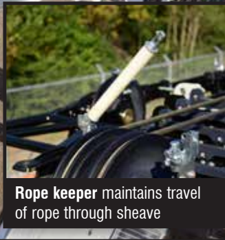
Quick reeve boom head eliminates the need to remove the becket when it becomes necessary to change the reeving
