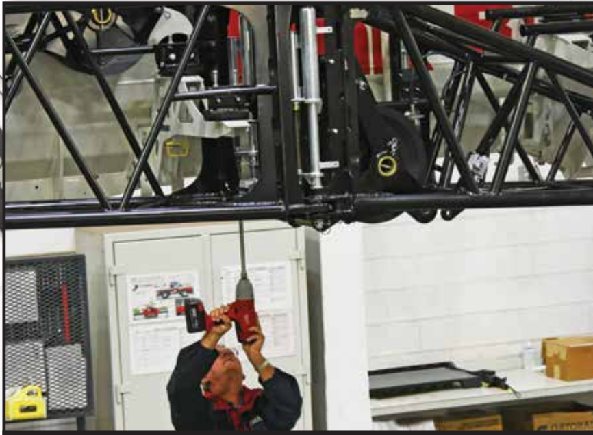
New efficient fly pinning design focuses on ease of assembly/disassembly
