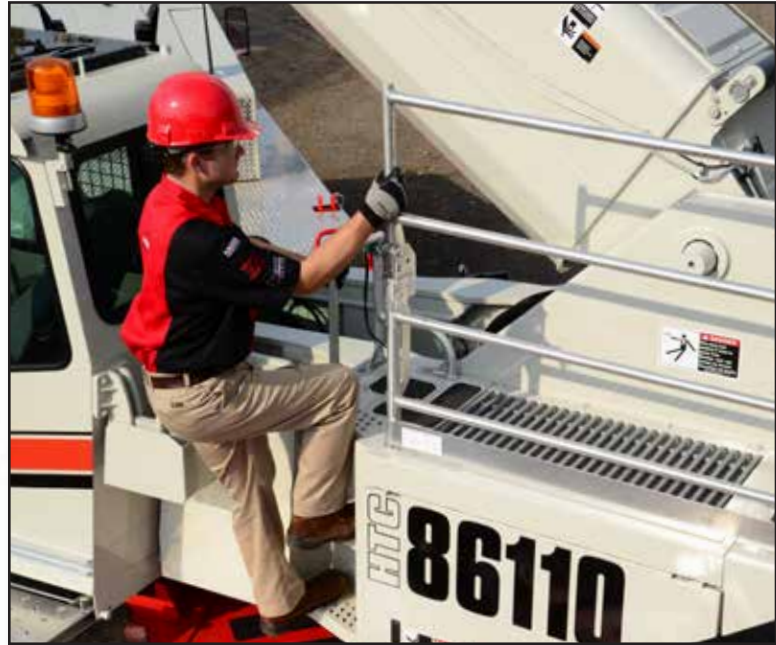
The upper work platform with folding handrails allows for easy inspection and maintenance of the HTC-86110.
