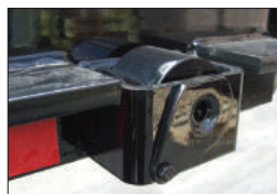
Removable side roller pin, secured by single bolt
