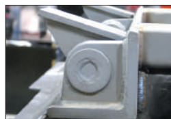
Hinge recessed into truck chassis, full width hinge shaft (1) piece construction
