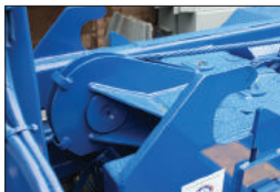
Larger 12" head sheave to improve cable life.
