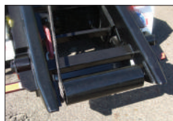
Full width rear roller reduces wear on tail
