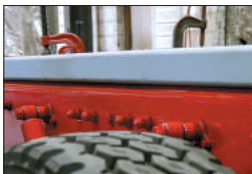
4" X 3" X 1/4" Flush mounted subframe
