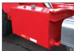
70 gallon hydraulic tank with side mounted brackets.
