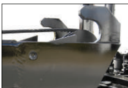
Dual spring loaded pull through front locks
