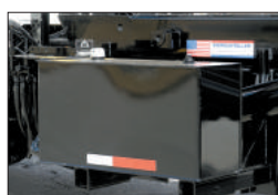
60 gallon hydraulic tank mounted on tubular bracket with dual filters
